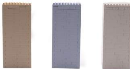
Three different dielectric materials with different dielectric constants and colours. The loss tangent is below 0,002.
